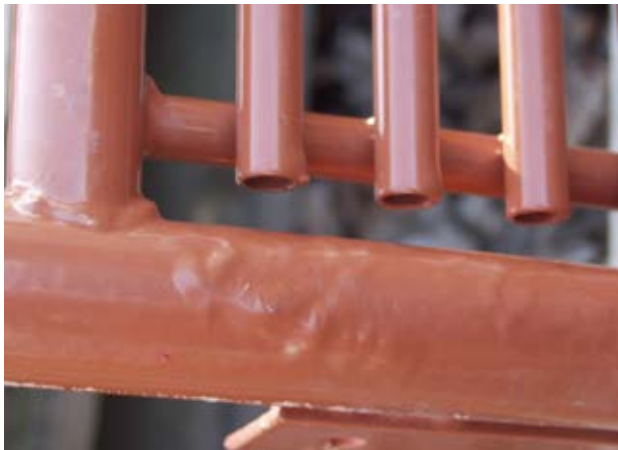
Figure 11: not-plastered zinc thickening
