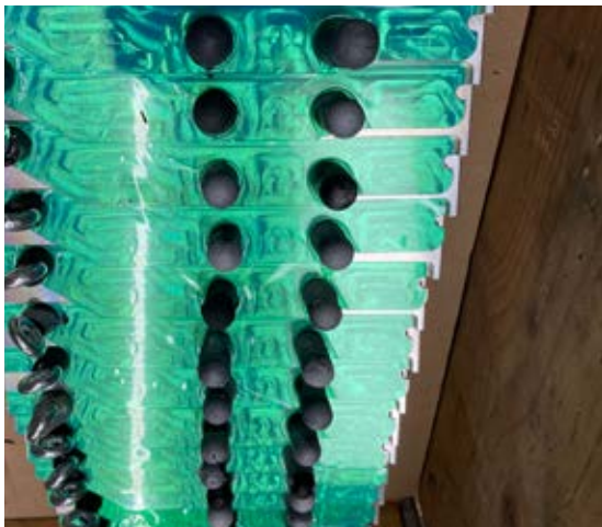
Figure 12: masked components before coating
