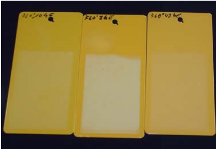
Figure 4: weathering stability, chalking
