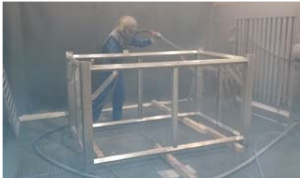
Figure 6 (left): Sandblasting in the open jet house
