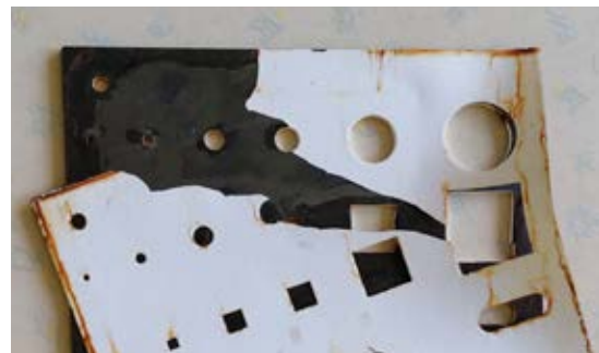
Figure 26: Test piece without edge rounding; full delamination after 250 h NSS
