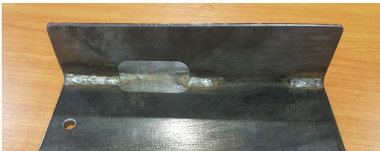
Figure 1: Welding foot: correct design on the left; risk of corrosion due to gap on the right
