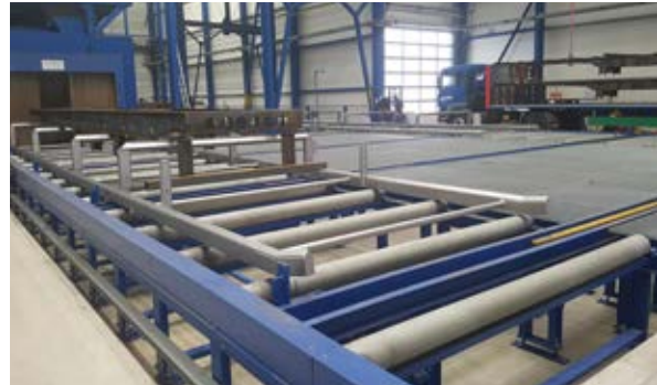
Figure 7 (right): Roller blasting unit
