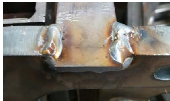
Figure 3 (right): Welded part with scale and grease burn-in
