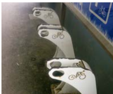
Figure 12: Bicycle stand with spalling and corrosion at the laser edge
