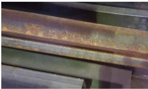
Figure 2 (left): Mill scale and corrosion on raw materials
