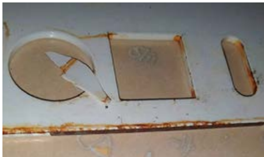
Figure 11: Test sheet with chipped coating on the laser edge
