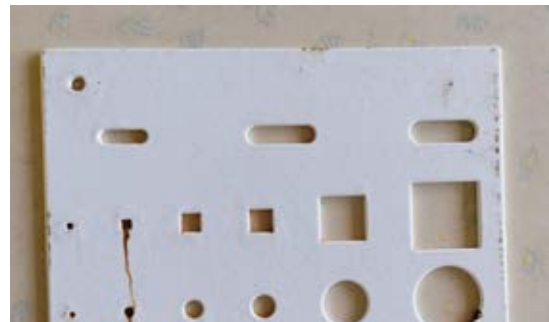
Figure 25: Test piece with rounded edges (0.5 mm); after 500 h NSS only minor signs of corrosion
