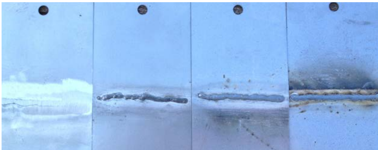
Figure 12: Weld seams in descending degree of cleaning
