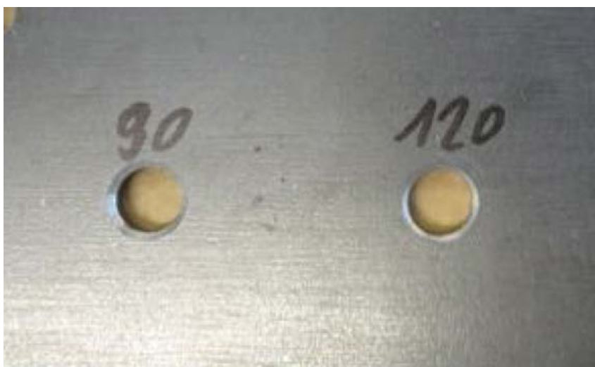
Figure 11: Special part of QIB project C5 with different prepared drilling holes, 90° lowered, 120° lowered
