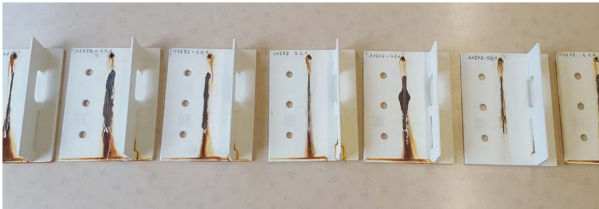
Figure 19: Overview of results of the QIB project C5 - test specimen after 1440 h neutral salt spray test from different coating companies
