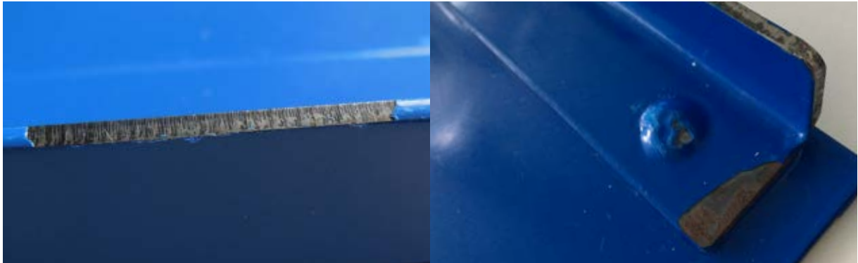
Figure 16: Unprocessed laser cutting edges with defects in corrosion and adhesion. The laser cuts are clearly visible. Oxide layers that form are sometimes difficult to remove by chemical pre-treatment. Laser systems working with inert gas can improve the situation.
