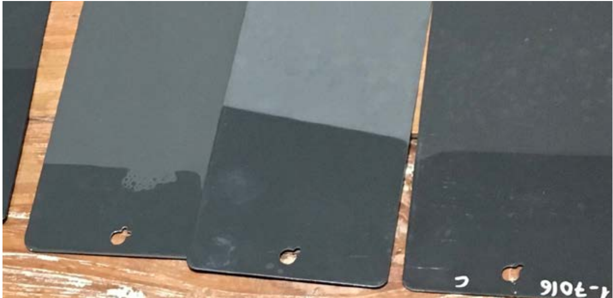
Figure 6: Moisture damage on powder-coated aluminium panels: Visible colour changes occur due to the storage of moisture.
