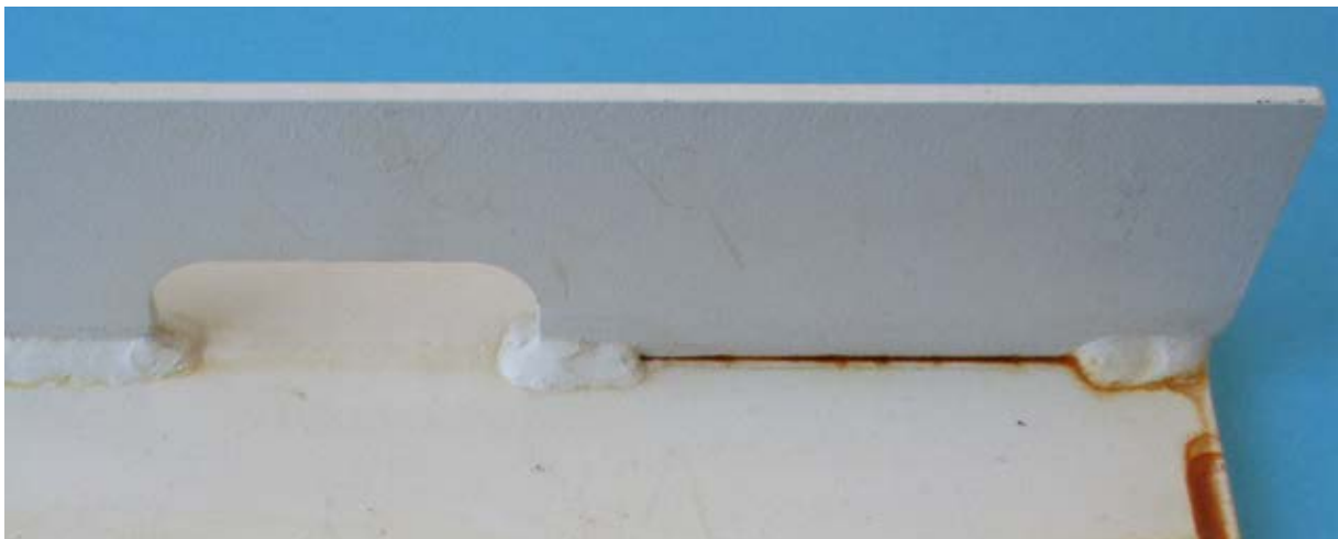
Figure 1: special test specimens of the QIB-project C5-2016 after 1440 h neutral salt spray testing DIN EN ISO 9227, note the corrosion appearance on the non-solid weld due to crevice corrosion.
