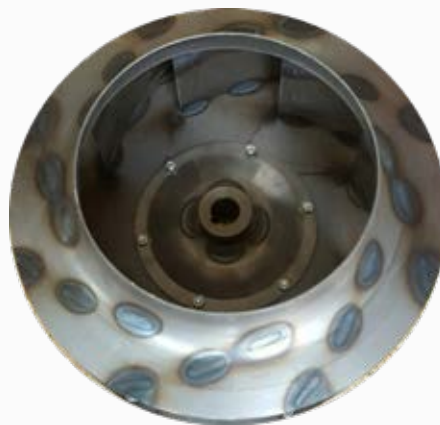
Figure 15: Component with a large number of HAZ shown during the presentation of the QIB project C5 (source: Bader Pulverbeschichtung GmbH)
