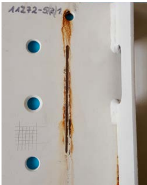
Figure 20: Detailed view of a sample that meets the currently valid standard requirements of a C5 corrosivity category. Corrosion visible in the gap could still be avoided by additional sealing.
