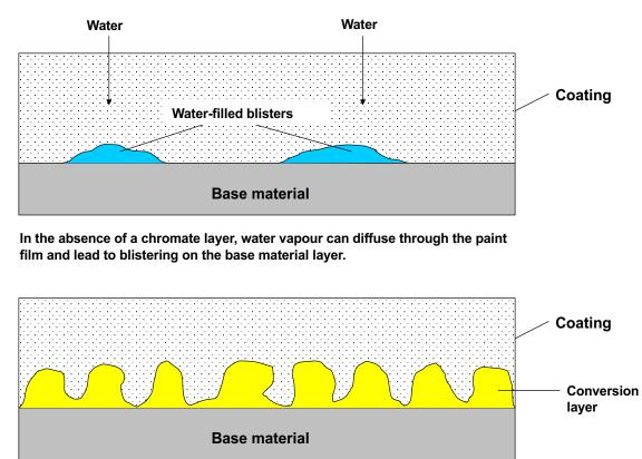
Here is the anchoring of the coating film in the conversion layer.
